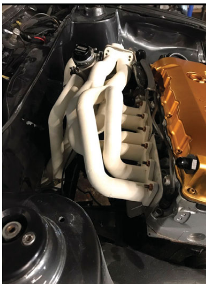
ABOVE B&B's thermal coatings are not just for protection, they also improve performance
