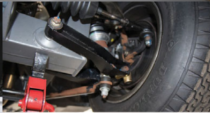
ABOVE The front suspension has trunnions to adjust the height, while the top wishbones are fully adjustable
